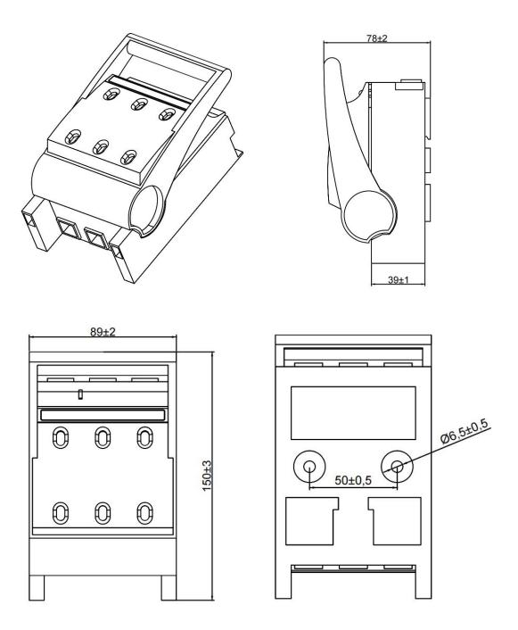
**CF-HR18** Fuse Switch Disconnector Dimension
