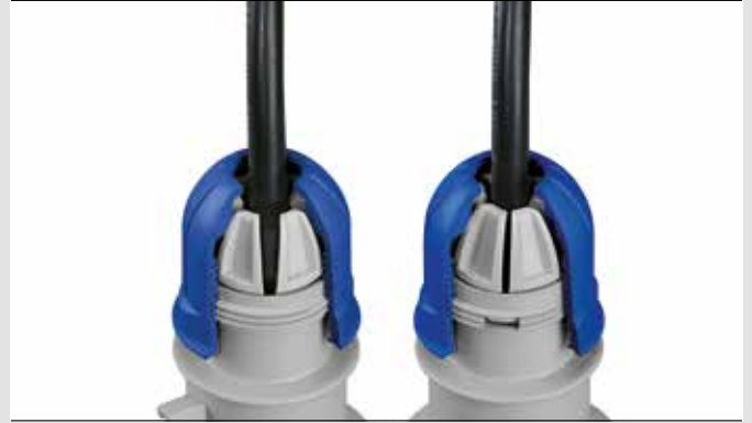
External cable stay with tulip clamping having IP66/IP67/IP69 cable gland functions (the device is used on both IP44/IP54 and IP66/IP67/IP69 products).
