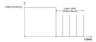
It is not recommended to prolong the duration of  $I_{\rm O}$  when it is <150% but >100%, since it may cause damage to the PSU.
