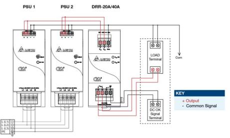
Fig. 3 Redundancy / Parallel Operation Connection Diagram
