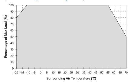
Fig. 1 De-rating for Vertical Mounting Orientation
