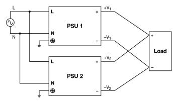
Fig. 4 Parallel Operation Connection Diagram
