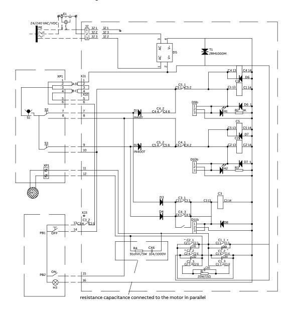
C1-C5 CONTACTOR MICRO SWITCH, START POSITION S1 POWER RESISTOR S2-S3 MICRO SWITCH, END POSITION R1 R2-R3 RESISTOR PB1 PUSHBUTTON ON/OFF R4 RESISTOR PB2 PUSHBUTTON ON/OFF D1-D4 DIODE E1 MINI CIRCUIT BREAKER D5 DIODE BRIDGE (not for 24 V) H1/H2 LIGHT DIODS D6-D8 DIODE Н3 CONTROL LAMP "DEVICE OK" XP1/XP2 TERMINATIONS FOR MOTOR Α CONNECTION FOR AUXITIAR SWITCH FOR XJ1-XJ3 TERMINATIONS FOR CONTACTOR UNIT **FUSEINTERRUPTION** Т1 DISCHARGE TUBE
