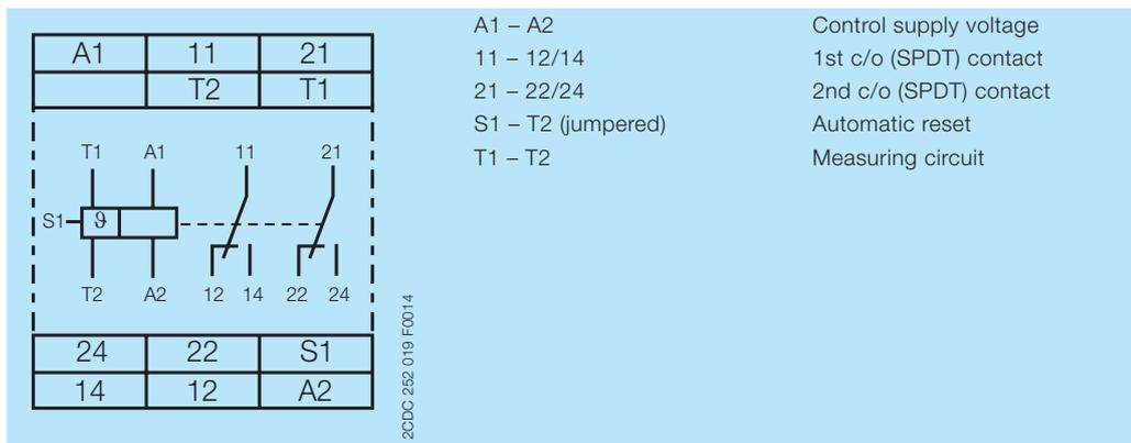
Connection diagram CM-MSS.41
