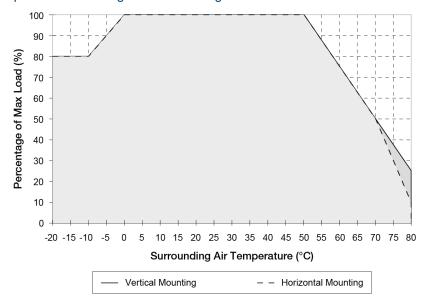
Fig. 1 De-rating for Vertical Mounting Orientation
